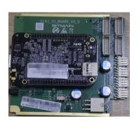
Integrated control board(A113D Control board), need to use the OTG cable (Micro usb - USB A)
